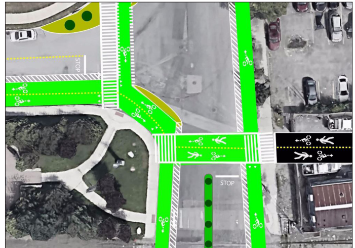
A plan view diagram from the 2018 Making The Case report shows the shared-use path transition from the railroad right-of-way to on-street bicycle infrastructure at the intersection of Inner Belt Road at New Washington Street and the dog park
